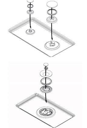
Assembly of the burner caps and burner grates
