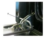
Insert an anti-rotation hinge in the appropriate holes. Hold the door by the sides and slowly close it until you can feel a certain resistance; now, while forcing the door closed, lift it in order to slide it out by freeing the hinge lock from the kitchen. To refit the door repeat the above instructions in reverse making sure the hinge lock is correctly fitted.
