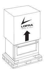
**IMPORTANT:** place the hand-truck straps below the oven door handles. To avoid damaging the side panels place a pad between the hand-truck and the range.
