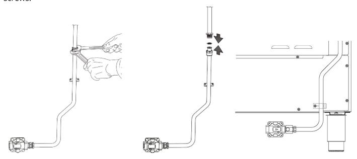
Take care to ensure the bracket is fitted the right way up with the opening at the top. The regulator cover must be oriented toward the front side of the range.
