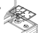
In the event of a momentary power failure, the hob burner can be ignited manually using an igniter.
